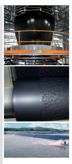
Bandera offer comprises complete extrusion lines with up to 1200 kg/h production capacity, with film thickness up to 3 mm
